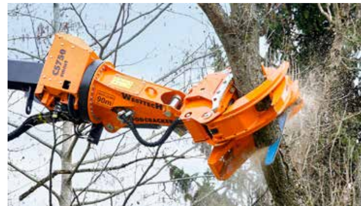
Woodcracker® CS750 flexHead² for tree care.
