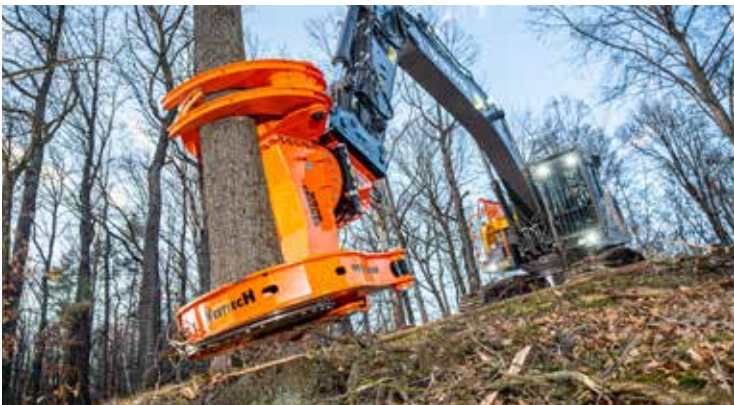
C650 with cutting diameter up to 70 cm.
