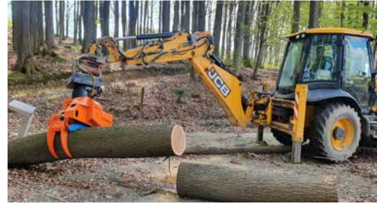
Sturdy and low-wear woodgripper with saw unit.
