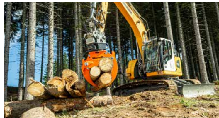
Gripper opening stroke 1270mm.
